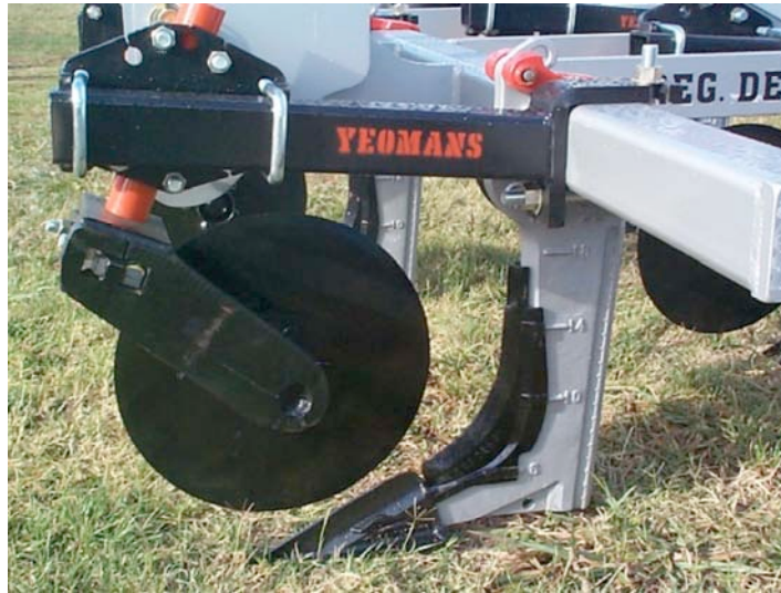
Figure 2. Yeomans Keyline plow shank with attached coulter.
